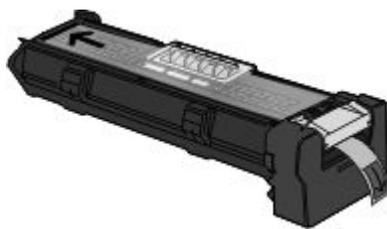
**6** Align and insert the end of the photoconductor.
