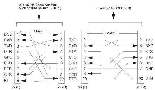
The following illustration shows the pin assignments for the 9-pin to 25-pin IBM EIA RS-232C serial cables.
