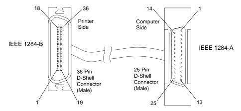
The following illustration shows the pin assignments for connecting the 25-pin connector to the 36-pin connector. The symbol \* indicates an active low signal.
