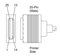
Pin assignments for this 25-pin connector are shown in Table 8-7. You can set the polarity of these signals from the printer operator panel or through MarkVision Professional.
