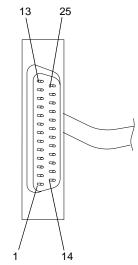
The following illustration shows the pin assignments for the 9-pin to 25-pin IBM EIA RS-232C serial cables.
