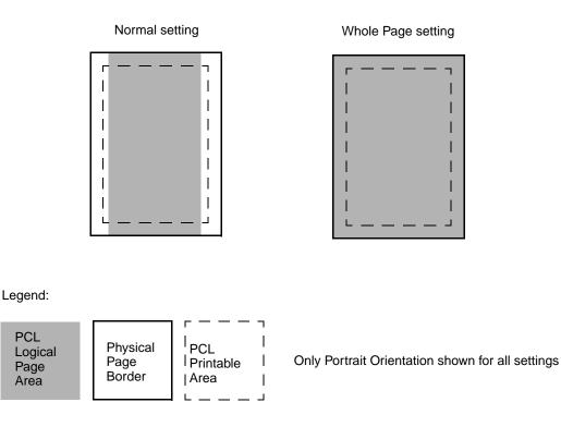
The *Normal setting*, which is the factory default, means the printable area includes the entire page except the narrow border around the edge of the page. This is the nonprintable area. The printer measures margin settings relative to the logical page.
