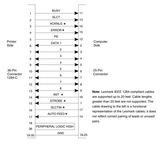
The following illustration shows the pin assignments for connecting the 25-pin connector to the 36-pin connector. The symbol \* indicates an active low signal.
