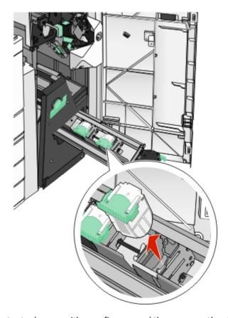
**6** Squeeze both sides of the empty staple case with your fingers, and then remove the staple case from the cartridge.
