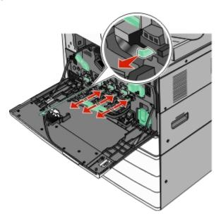
Slide the printhead wipers back into place.
