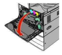
**2** Rotate the release lever counterclockwise to open the cover.
