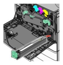
Rotate the release lever counterclockwise to open the cover.
