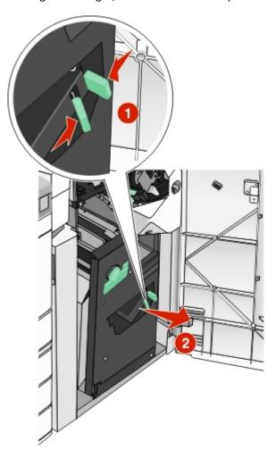
**3** Hold the tabs on both sides of the staple cartridge.
