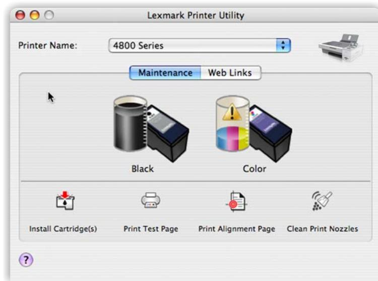
If an exclamation point (!) appears on a cartridge, the ink level is low. Install a new cartridge.
