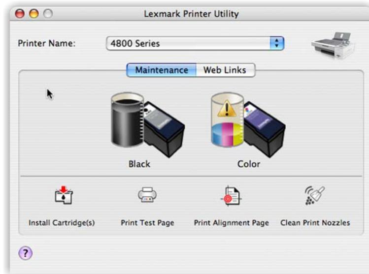
If an exclamation point (!) appears on a cartridge, the ink level is low. Install a new cartridge. For more information, see “Installing print cartridges” on page 95.
