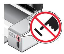
**Note:** The printer recognizes one active media device at a time. If you insert a flash drive and a memory card, the  $\circlearrowleft$  light and the  $\stackrel{\cong}{=}$  light blink alternately until either the memory card or flash drive is removed.
