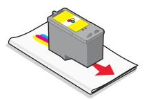
**4** Using another clean section of the dampened cloth, gently hold the cloth against the contacts for about three seconds, and then wipe in the direction shown.
