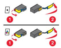
3 Reinstall the cartridges.
