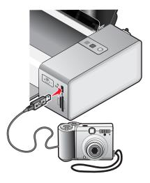
**Warning:** Do not touch the USB cable, any network adapter, or the printer in the area shown while actively printing from a PictBridge-enabled digital camera. A loss of data can occur. Also, do not remove the USB cable or network adapter while actively printing from a PictBridge-enabled digital camera.
