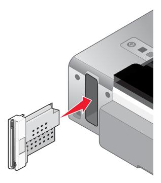
**Warning:** Wireless print servers are easily damaged by static electricity. Touch something metal such as the printer frame before you touch the wireless print server.
